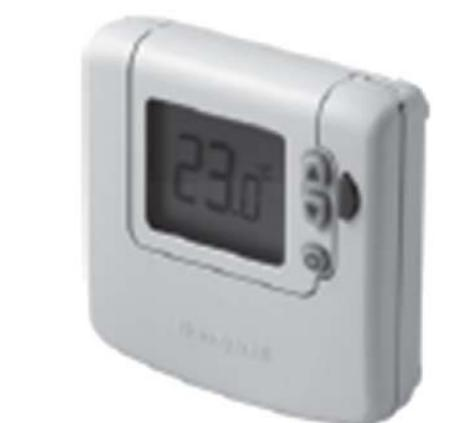
The thermostat in the living room sets the temperature in the room. 20-21°C is the normal temperature, but you could turn it down if you go away for a few days. The thermostat buttons include a green eco button which turns the temperature down for a few hours, say when you want to go out, but this is not necessary.
