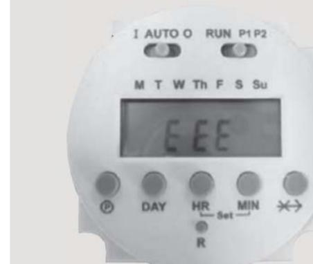
The timer on the boiler controls the heating on/off periods. This should be set for all-day-long because the ventilation system is designed to provide gentle continuous heat. It can't give a quick boost like radiators can.
